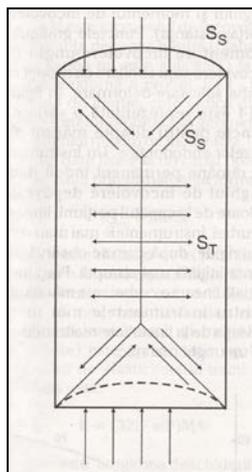
**Fig.6 Drawing of complex stress pattern developed in cylinder subjected to compressive stress.. (after, Craig R.. and colab, 2001)**
