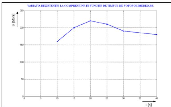
**Fig.5 The graphical expression of the compression strength variation of the composite materials specimens according to the light-curing time**
