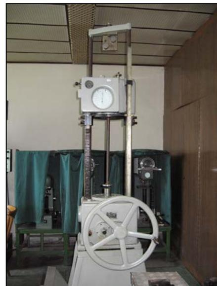
**Fig.4 The Universal Testing Machine for mechanical properties with a gamma from 0 to 1000kgF and a gradation of 2 kg**
