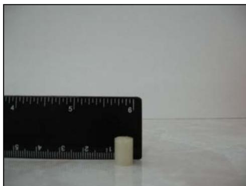
**Fig.1 and 2 The specimens of light-curing composite material with 5 mm diameter and 10 mm height**
