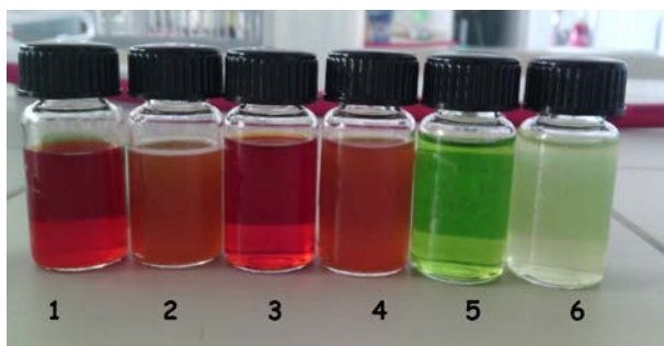
Fig.2. Ultrasonicated extracts: 1- Capsicum annuum (red variety, ethanolic extract); 2- Capsicum annuum (red variety, aqueous extract); 3- Capsicum annuum without seeds and ribs (red variety, ethanolic extract); 4- Capsicum annuum without seeds and ribs (red variety, aqueous extract); 5- Capsicum annuum (green variety, ethanolic extract); 6- Capsicum annuum (green variety, aqueous extract);
