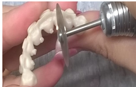
Fig.5. Adjusting sintered zirconia framework
