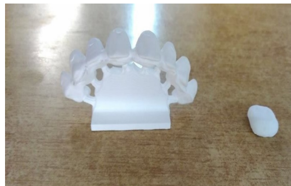
Fig.4. Oversized zirconia framework before sintering
