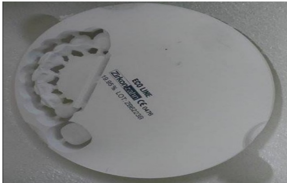
Fig.3. Zirconia milled framework
