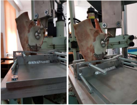
Figure 11. Assembly with a morcellated bone graft attached to the EDZ 20 test machine.
